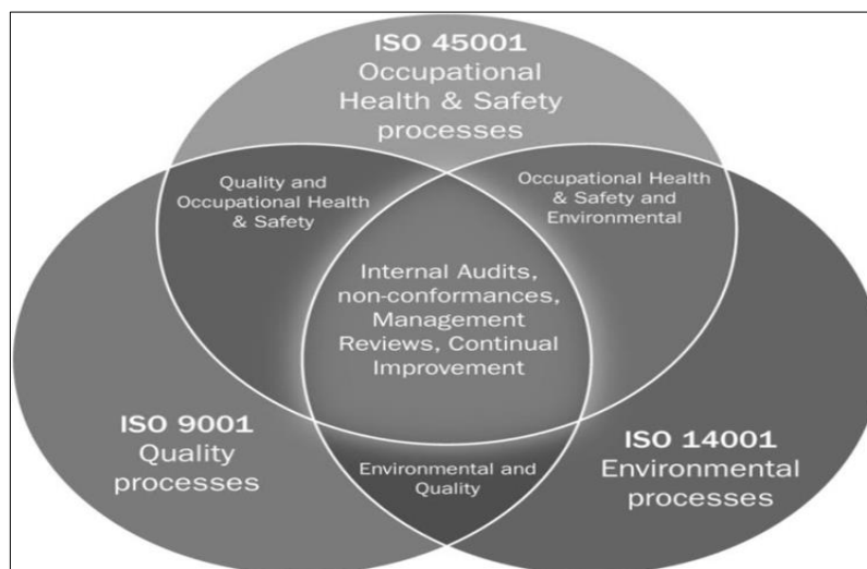
Figure 11: The integration of the QMS, EMS and OHSMS according to ISO 9001:2015, ISO14001:2015 and ISO 45001: 2018 standards.
