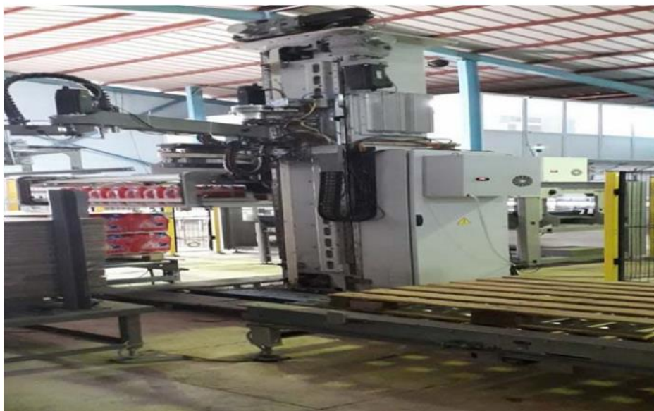
Figure 11: the robotic palletiser
