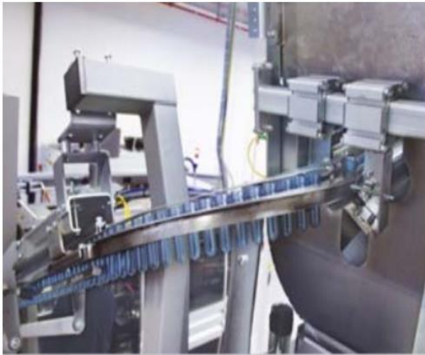
Figure 8: Preform feeding unit
