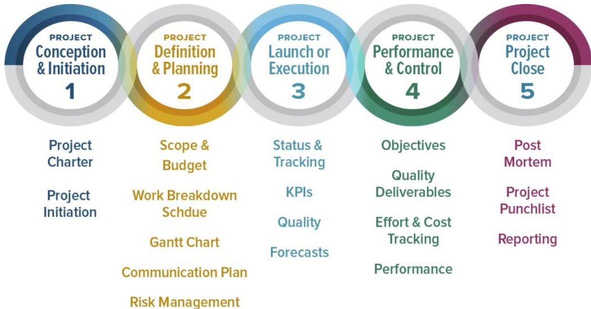
Figure 4: Five (5) Phases of a Project
